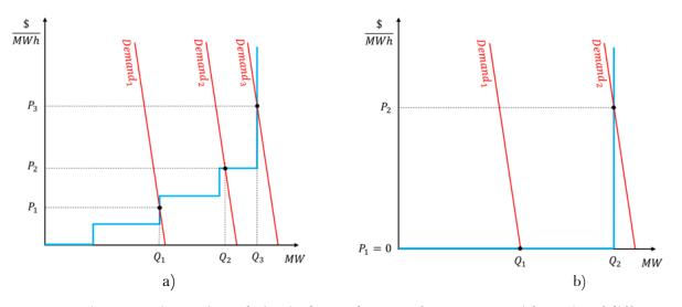
Figure 1: a) Supply and elastic demand curves for a system with a mix of different conventional generation units, b) Supply and elastic demand curves for a system where all units have zero marginal cost.
